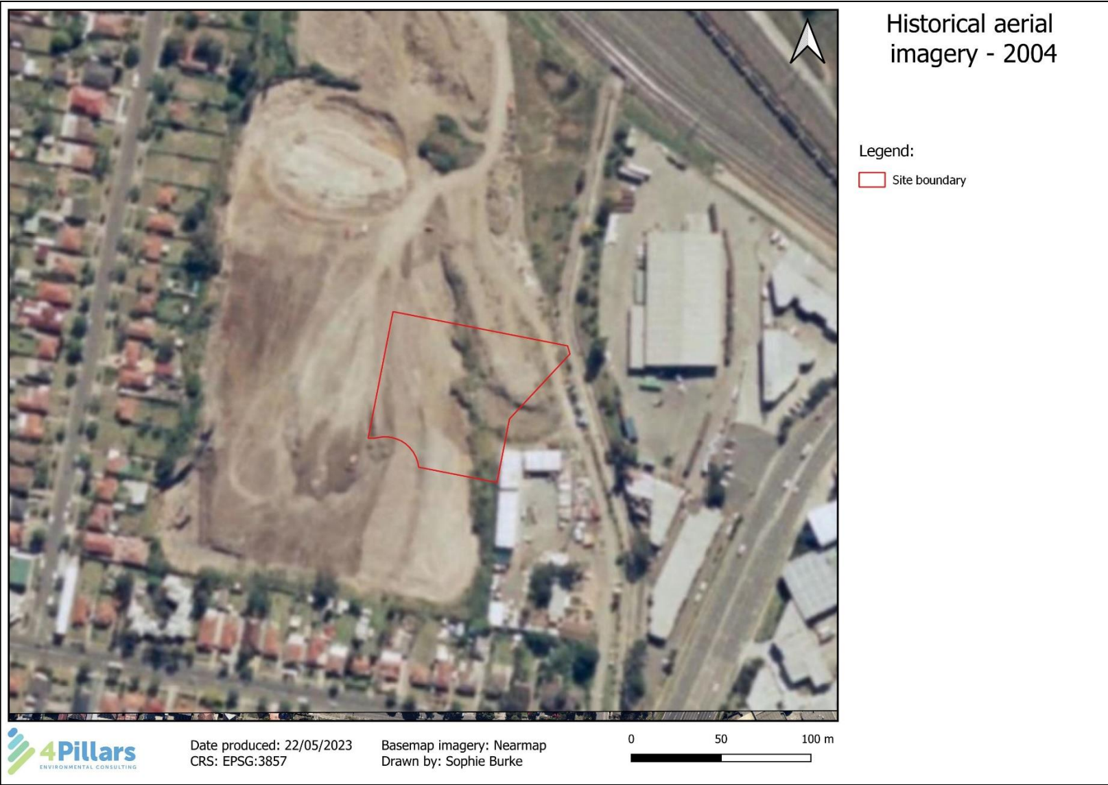
Figure 13: Historical aerial imagery 2004, showing the quarry void being filled with soil materials.
